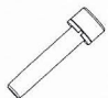
29 Hexagon socket head spring washer combination screw M5X25 x 4 内六角圆柱头弹垫组合螺钉 M5X25
